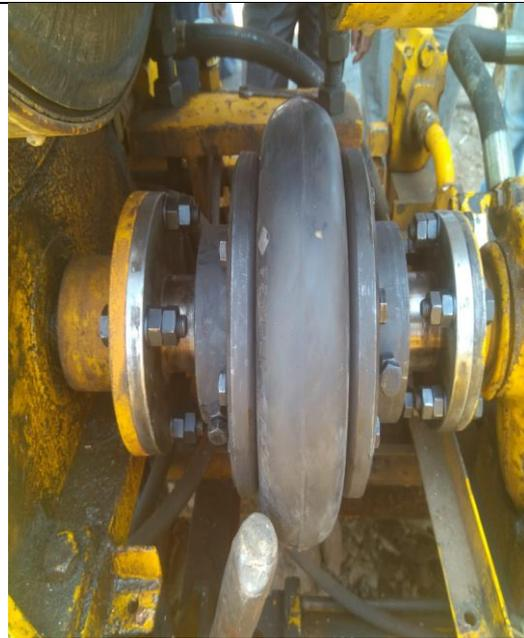
**Present Modified Coupling in the drilling rig**
