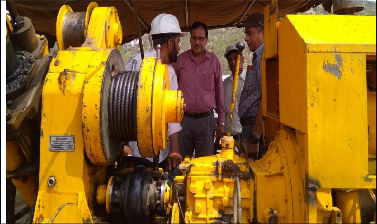
**Shri Brij Kumar, ADG & HOD, GSI, WR inspecting the drilling rig with Modified Coupling**
