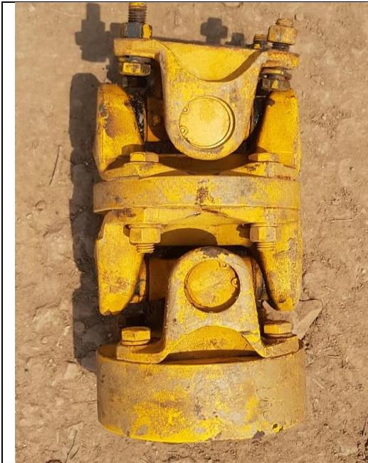
**Originally Fitted Coupling in the drilling rig**
