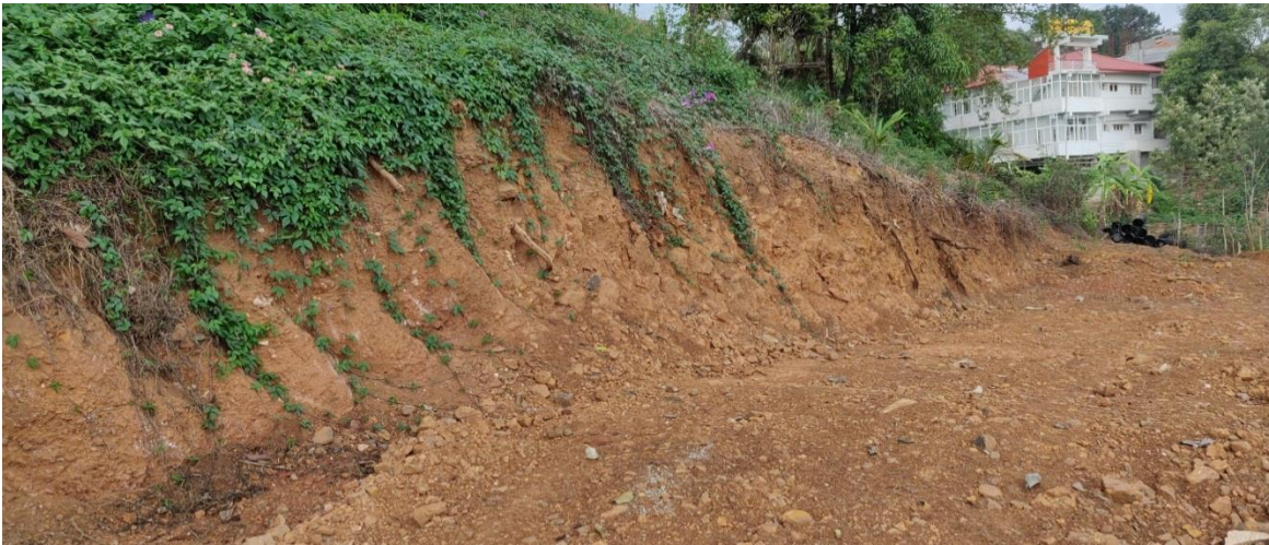
Photo – 4: View of weathered granite gneiss exposed at the top of the hill slope.
