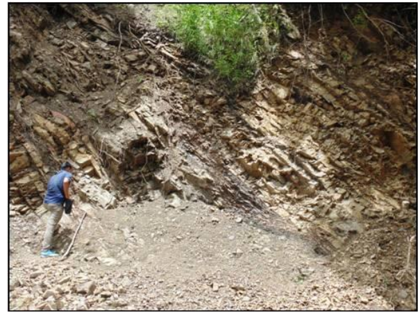
Fig. 7: Photograph showing highly jointed and weathered shale - siltstone - sandstone intercalation at the site of the landslide.
