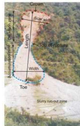
Fig 1.2 Left figure: a simplified illustration of a rotational landslide (earth slide) that evolved into earth flow. Image illustrates commonly used labels for the parts of a landslide (from Varnes, 1978); Right figure: annotated photograph showing important landslide features. Red and blue lines represent landslide initiation and deposition area, respectively.
