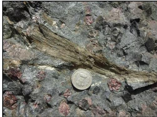
Field Photograph showing formation of garnet (red colour), gahnite, anthophyllite (brown colour, broom shape) and chlorite mineral assemblages zone (defined as alteration mineralogy) at Borgaon -Tarora (22° 15' 30":: 78° 14' 20") is represented as standard alteration assemblages as a result of Hydrothermal alteration zone developed along the VMS deposits of Betul Belt.
