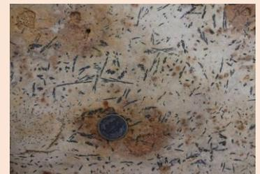
Field Photograph showing porphyritic texture in rhyolite with development of randomly oriented needle shape hornblende phenocryst set in the fine grained quartz-feldspar matrix at Jilardev (22° 18' 29" :: 78° 35' 46").
